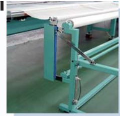
Fabric serpentine feed preventing mechanism Fabric is fed in the stretched conditions to realize stabilized fabric feed, free from serpentine.
